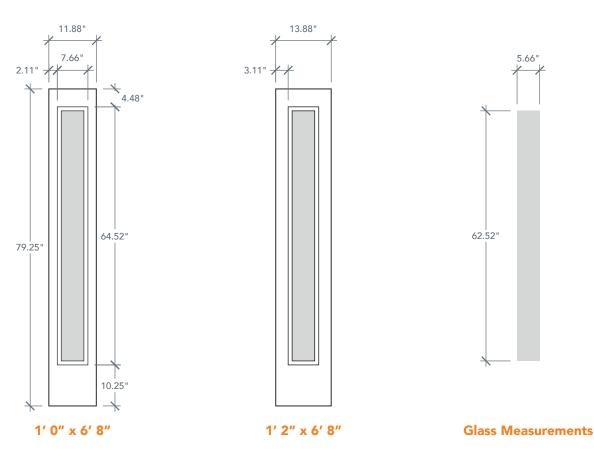
NOTE: BY REQUEST, SIDELITE HEIGHT COMES IN VARYING DIMENSIONS TO A MINIMUM OF 79". EXCESS WILL BE TAKEN FROM BOTTOM RAIL. ALL OTHER DIMENSIONS WILL REMAIN THE SAME.
