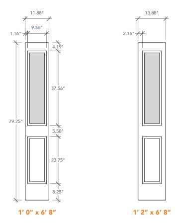
NOTE: BY REQUEST, SIDELITE HEIGHT COMES IN VARYING DIMENSIONS TO A MINIMUM OF 79". EXCESS WILL BE TAKEN FROM BOTTOM RAIL. ALL OTHER DIMENSIONS WILL REMAIN THE SAME.
