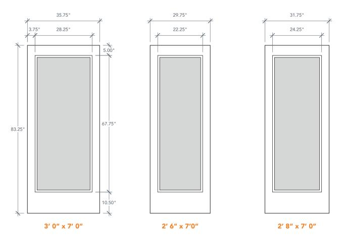
NOTE: BY REQUEST, DOOR HEIGHT COMES IN VARYING DIMENSIONS TO A MINIMUM OF 83". EXCESS WILL BE TAKEN FROM BOTTOM RAIL. ALL OTHER DIMENSIONS WILL REMAIN THE SAME.
