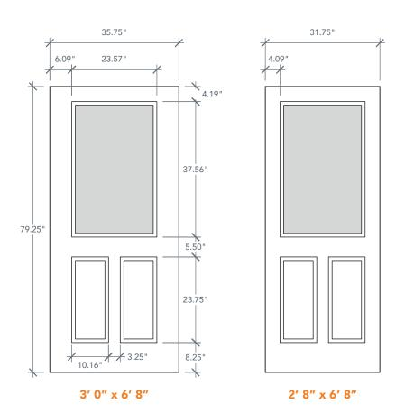
NOTE: BY REQUEST, DOOR HEIGHT COMES IN VARYING DIMENSIONS TO A MINIMUM OF 79". EXCESS WILL BE TAKEN FROM BOTTOM RAIL. ALL OTHER DIMENSIONS WILL REMAIN THE SAME.
