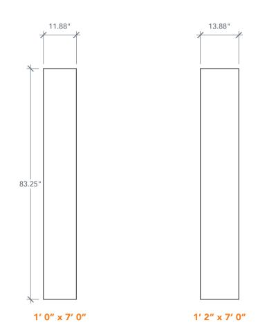
NOTE: BY REQUEST, SIDELITE HEIGHT COMES IN VARYING DIMENSIONS TO A MINIMUM OF 83". EXCESS WILL BE TAKEN FROM BOTTOM RAIL. ALL OTHER DIMENSIONS WILL REMAIN THE SAME.
