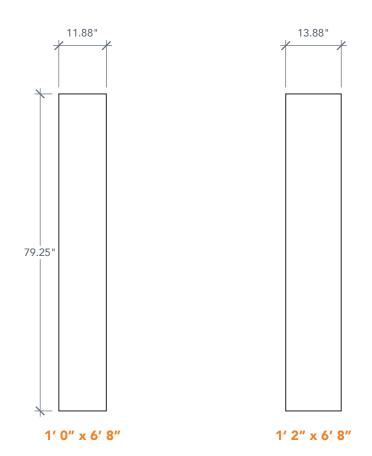
NOTE: BY REQUEST, SIDELITE HEIGHT COMES IN VARYING DIMENSIONS TO A MINIMUM OF 79". EXCESS WILL BE TAKEN FROM BOTTOM RAIL. ALL OTHER DIMENSIONS WILL REMAIN THE SAME.
