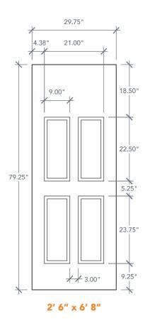
NOTE: BY REQUEST, DOOR HEIGHT COMES IN VARYING DIMENSIONS TO A MINIMUM OF 79". EXCESS WILL BE TAKEN FROM BOTTOM RAIL. ALL OTHER DIMENSIONS WILL REMAIN THE SAME.
