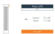
NOTE: BY REQUEST, SIDELITE HEIGHT COMES IN VARYING DIMENSIONS TO A MINIMUM OF 79". EXCESS WILL BE TAKEN FROM BOTTOM RAIL. ALL OTHER DIMENSIONS WILL REMAIN THE SAME.
