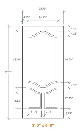
NOTE: BY REQUEST, DOOR HEIGHT COMES IN VARYING DIMENSIONS TO A MINIMUM OF 79". EXCESS WILL BE TAKEN FROM BOTTOM RAIL. ALL OTHER DIMENSIONS WILL REMAIN THE SAME.
