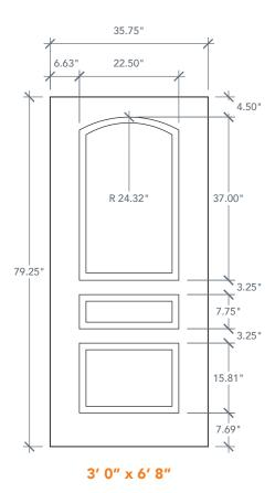
NOTE: BY REQUEST, DOOR HEIGHT COMES IN VARYING DIMENSIONS TO A MINIMUM OF 79". EXCESS WILL BE TAKEN FROM BOTTOM RAIL. ALL OTHER DIMENSIONS WILL REMAIN THE SAME.
