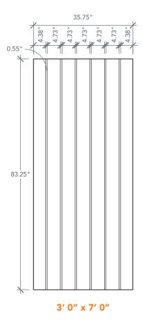
NOTE: BY REQUEST, DOOR HEIGHT COMES IN VARYING DIMENSIONS TO A MINIMUM OF 83". EXCESS WILL BE TAKEN FROM BOTTOM RAIL. ALL OTHER DIMENSIONS WILL REMAIN THE SAME.
