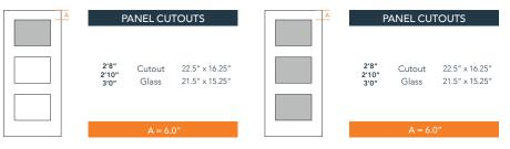
A = DISTANCE FROM TOP OF DOOR TO TOP OF OPENING. NOTE: PLASTPRO DOES NOT PROVIDE PRE-CUT CONFIGURATION SERVICE FOR THIS DOOR. ADD-IN LITE FRAME AVAILABLE IN SOLUTION DOORLITE SERIES.
