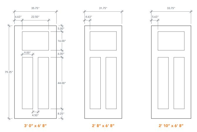
NOTE: BY REQUEST, DOOR HEIGHT COMES IN VARYING DIMENSIONS TO A MINIMUM OF 79". EXCESS WILL BE TAKEN FROM BOTTOM RAIL. ALL OTHER DIMENSIONS WILL REMAIN THE SAME.
