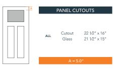
A = DISTANCE FROM TOP OF DOOR TO TOP OF OPENING. NOTE: PLASTPRO DOES NOT PROVIDE PRE-CUT CONFIGURATION SERVICE FOR THIS DOOR. ADD-IN LITE FRAME AVAILABLE IN SOLUTION DOORLITE SERIES.
