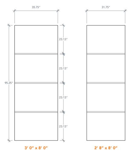
NOTE: BY REQUEST, DOOR HEIGHT COMES IN VARYING DIMENSIONS TO A MINIMUM OF 95". EXCESS WILL BE TAKEN FROM BOTTOM RAIL. ALL OTHER DIMENSIONS WILL REMAIN THE SAME.
